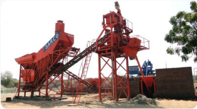
Concrete Batch Plant (Halla Hagon) 45 CM/Hr.
