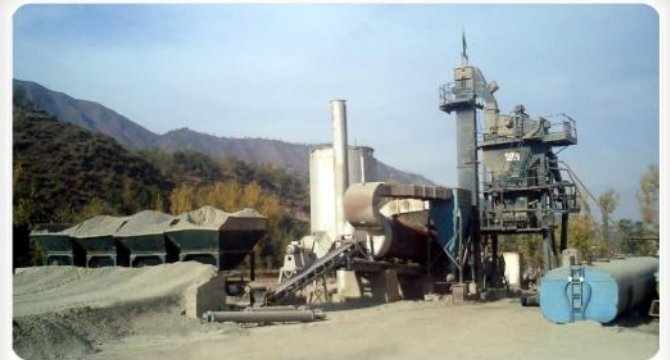
Asphalt Plant Parker England (80/100 Ton/Hr) Working at Gujrat
